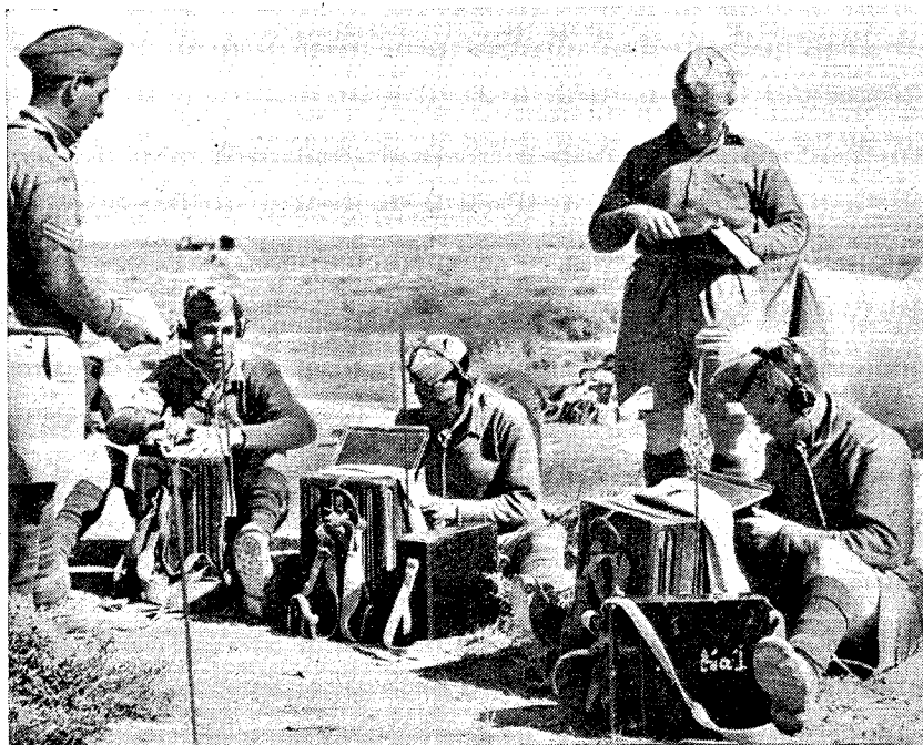
TRAINING infantrymen of the 8th Army in the use of the No. 18 set. The case beside each set is the heavy-duty "static" battery which is used for non-mobile purposes.
